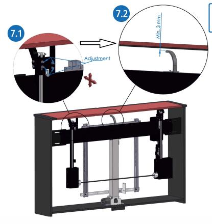
Minimum free space between the lifts top part and cover is 3 mm.
